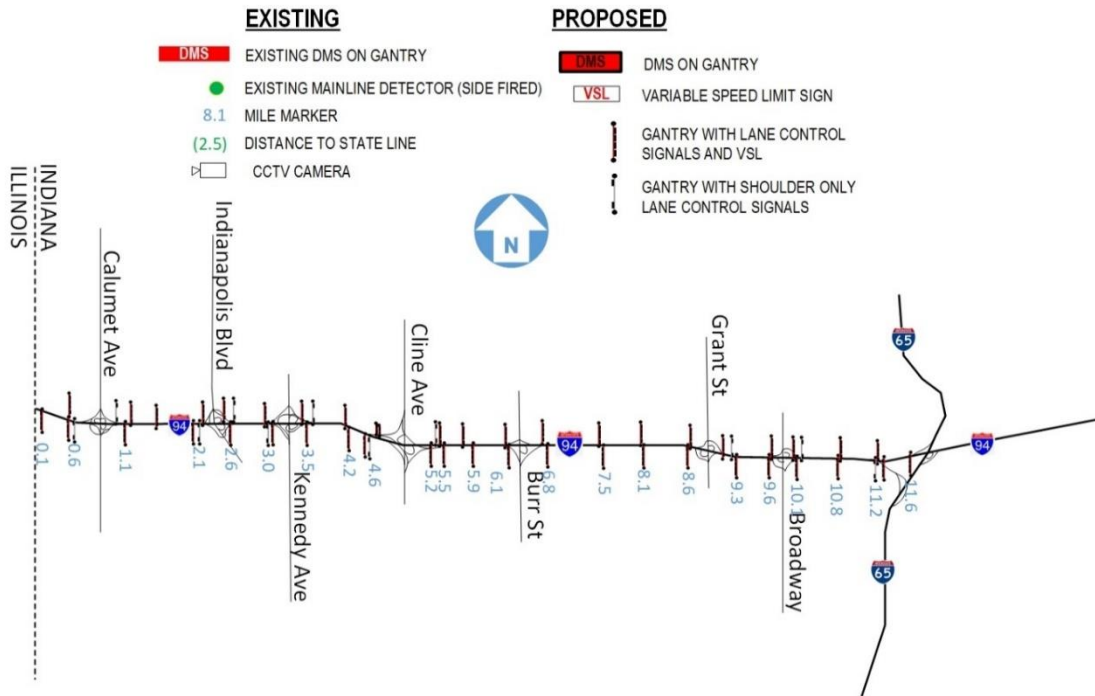
Figure 4.8: Preliminary Lane Control Signal Gantry Locations in Indiana
